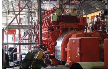
GE's Waukesha 12V 275GL+ engines drive pumps to transport NGLs from the jungles of Peru. The engine is shown here in a packaging facility in Mendoza, Argentina, ready for a string test.
